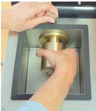
Mounting of the test-bearing housing with snap-closure arresting pin
